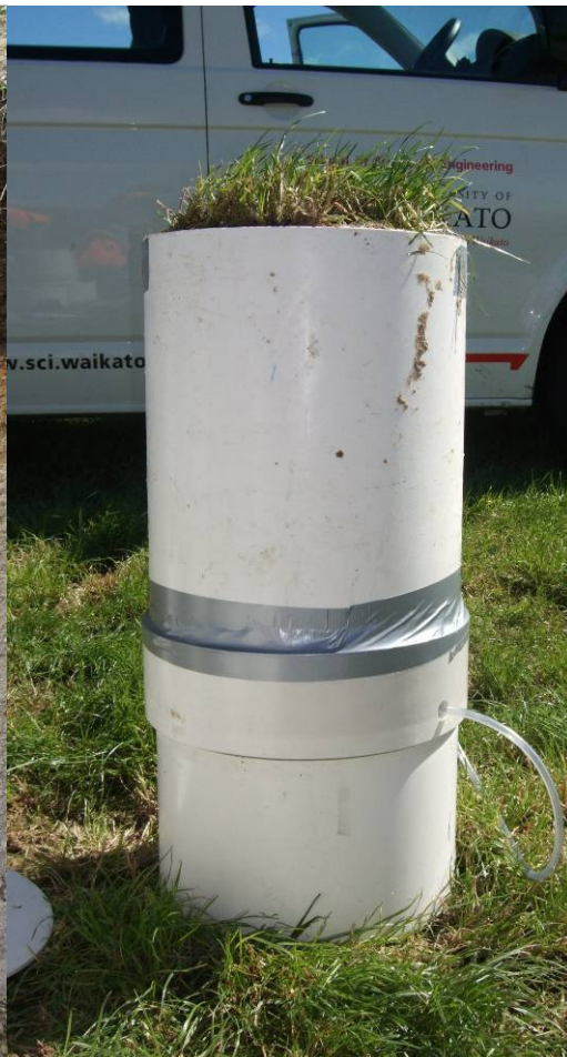
Figure 2. Lysimeter ready for installation, note leachate collection chamber with sampling hose.
